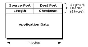
The UDP transport service adds to IP the ability to deliver a datagram to a specified destination process using a port abstraction, in an analogous way to that used by TCP.
